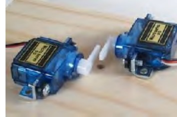
2-12: Tam Valley Depot's Dual 3-Way semaphore driver and typical servo mechanisms.
