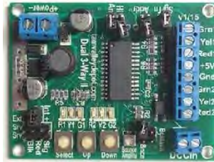
2-12: Tam Valley Depot's Dual 3-Way semaphore driver and typical servo mechanisms.
