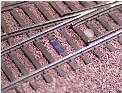
2-6: Optical sensors: IR integrated (left) and ambient (right).
