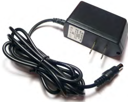
2-15: Wall-wart style AC power supply.
