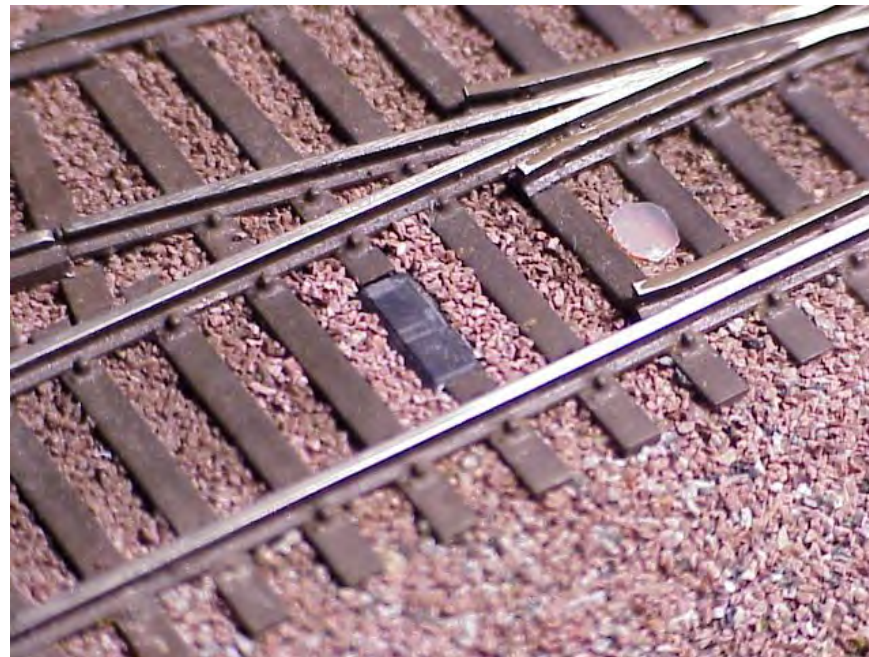
1-17: Track-mounted optical sensors. Infrared reflective (left) and ambient (right).
